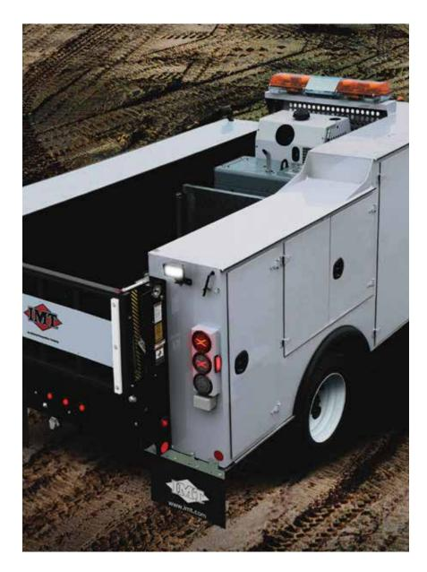
often performed by LED lamps, while backup lighting remained largely the realm of incandescent lamps. Optronics' Fusion LED combination stop, tail, turn, and backup lamps were designed to give users the benefit of two lamps for the price of one. Additionally, because the lamps are LED, they are more dependable and safer than incandescent lamps.
