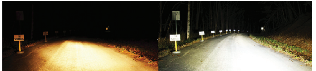
LED headlamps provide a better view for the driver because the light emitted is in a color spectrum which provides high contrast and is more readily seen by the eye. The left photo shows the illumination from halogen headlamps at low beam. The right photo shows LED headlamps at low beam.
