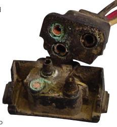
tect against moisture and debris," Truck-Lite's Liuzzo says. "Fleets should also immediately stop using any wire probes to test system voltage or continuity. Piercing the wire with a probe will allow moisture to run through the harness, corroding the system from the inside out."
