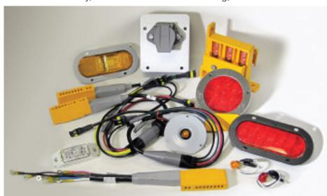
repairs should always be done with sealed terminals," he says. "We recommend the use of bare terminals that are protected by quality dual wall heat shrink that utilizes some sort of sealing compound to make them truly weatherproof."
