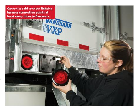
any corrections that are necessary to stop further corrosion, and then reapply new dielectric grease to it before mating it back together again."
